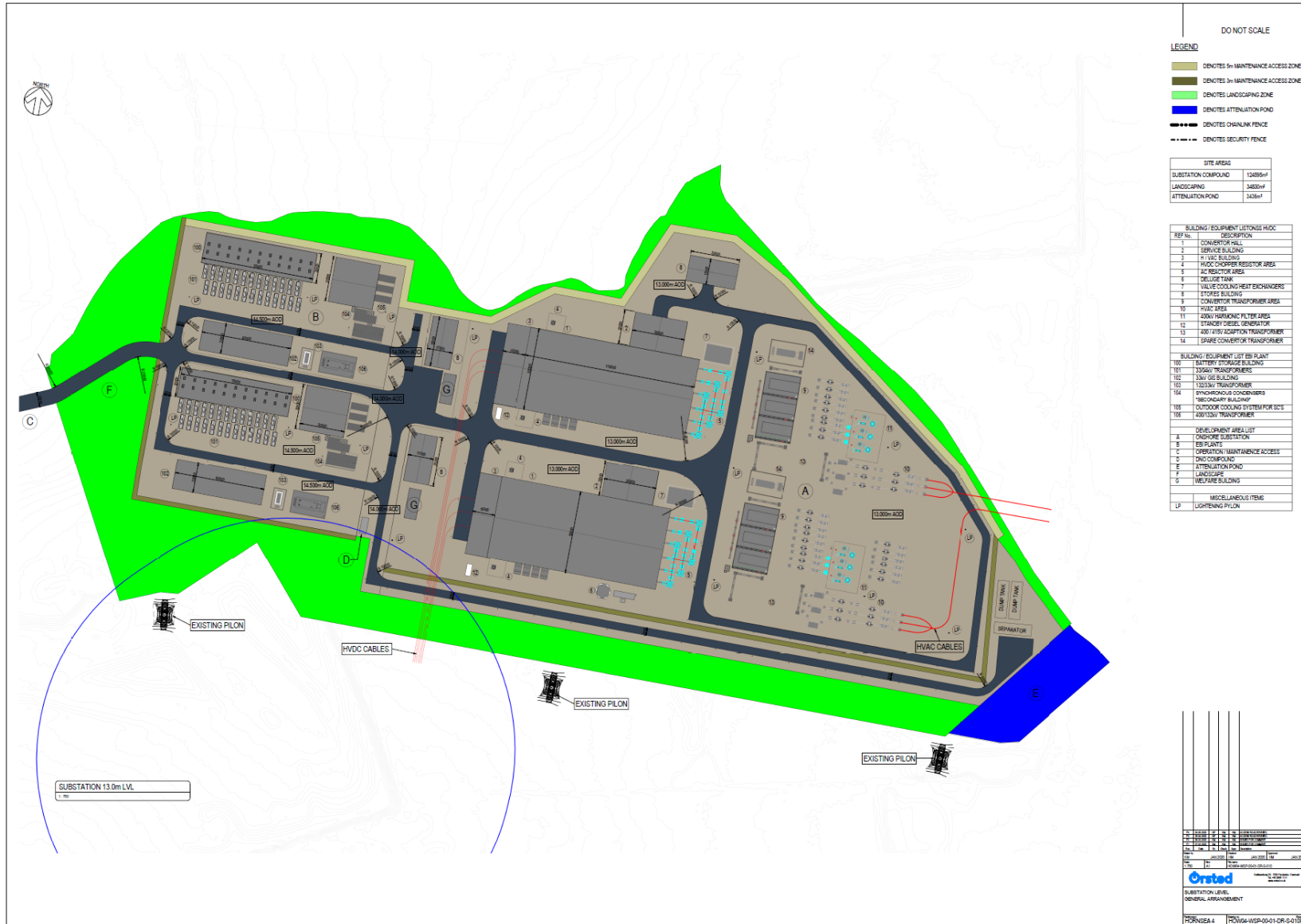
Figure 4: Indicative HVDC OnSS and EBI Layout.
